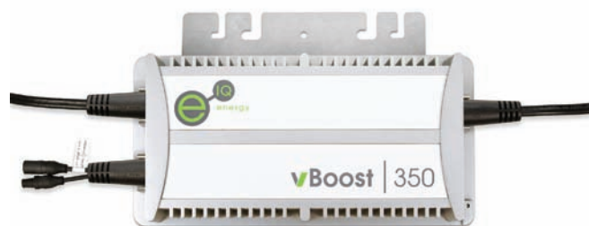
eIQ Parallax vBoost units raise voltage and are wired in parallel to capture maximum power. Because these units can accept up to 350 W, more than one module can be wired to each unit.
